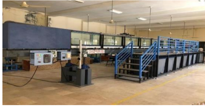
Figure 2: Computerized Flow Channel
