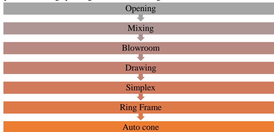
Figure 1: Flow Chart Ring Spinning Process
